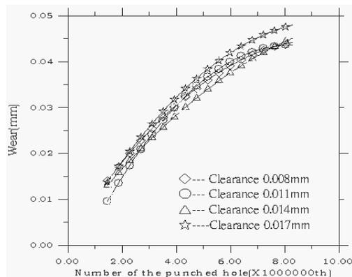
Fig. 14. The relationship between number of the punched hole and wear of punch BO-side
