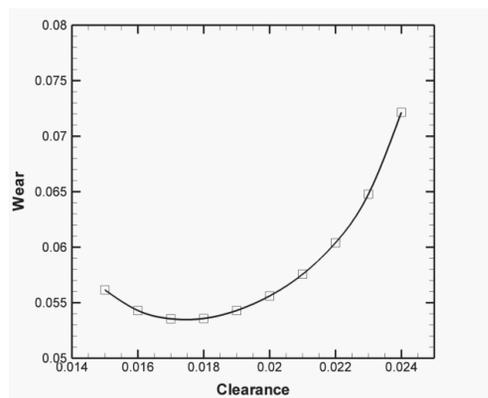
Fig. 17. The relationship between clearance and wear of punch AO-side
