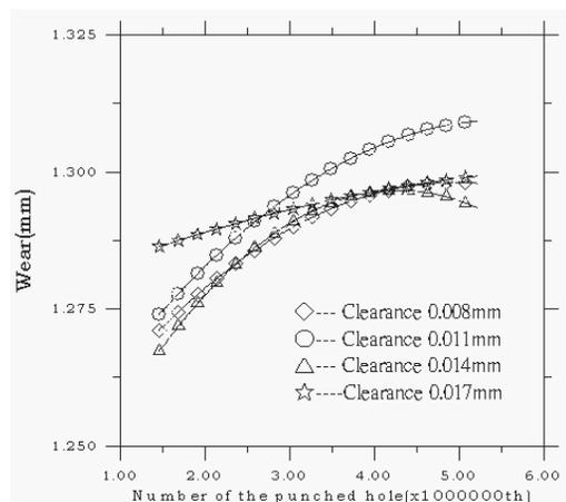
Fig. 16. The relationship between number of the punched hole and wear of die AO-side
