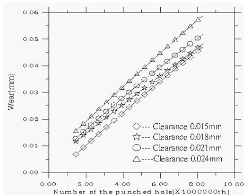
Fig. 13. The relationship between number of the punched hole and wear of punch AO-side
