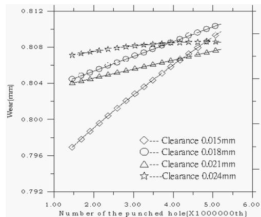
Fig. 15. The relationship between number of the punched hole and wear of die AO-side
