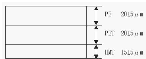
Fig. 2. The experimental composite
