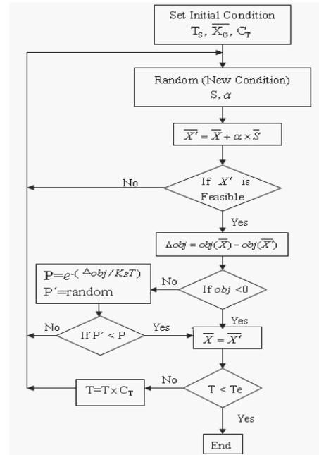
Fig. 12. The flow chart of SA method
