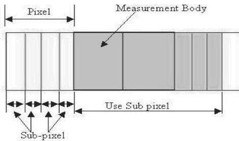
Fig. 9. Sub-pixel measurement
