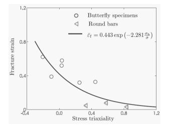
Fig. 10. Calibrated fracture locus of the present AC4CH-T6 cast aluminum alloy
