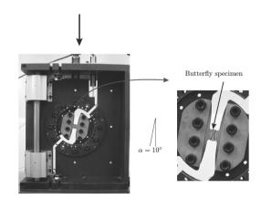
Fig. 4. A butterfly specimen with the orientation angle of 10 degree mounted in the Universal Biaxial Testing Deice (UBTD)
