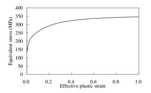
Fig. 7. The true stress-strain curve for the present cast aluminum alloy with the elastic modulus of 86.0 GPa and the Poisson's ratio of 0.33
