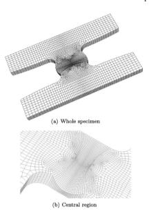
Fig. 6. Finite element model of the butterfly specimen
