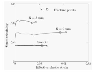
Fig. 8. Evolution of the stress triaxiality and the effective plastic strain of the critical material points for the round bar specimens
