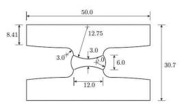
Fig. 3. Major dimensions of the butterfly specimen (unit: mm)
