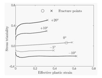
Fig. 9. Evolution of the stress triaxiality and the effective plastic strain of the critical material points for the butterfly specimens
