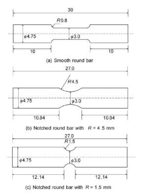
Fig. 2. Dimension of the round bar specimens (unit: mm)
