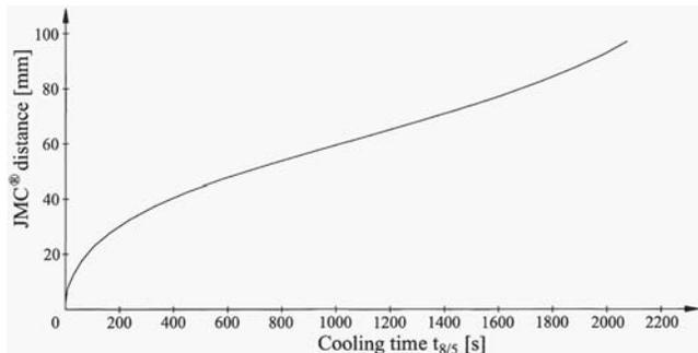
Fig. 4. Distance from the quenched end of JMC<sup>®</sup>-specimen vs. cooling time  $t_{8/5}$
