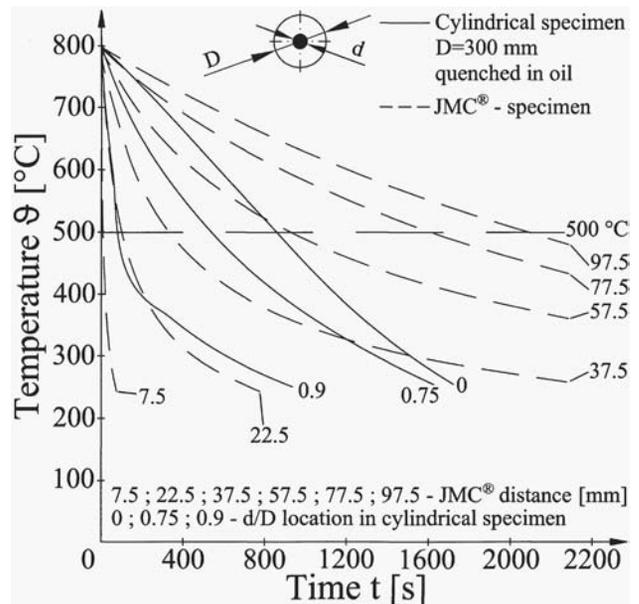
Fig. 5. Cooling curves of cylindrical specimen (D=300 mm)
