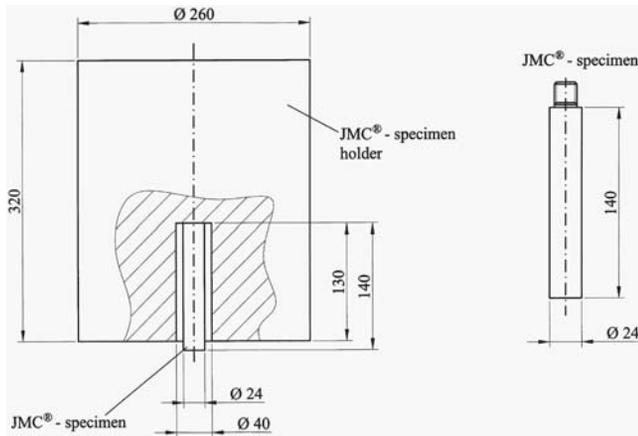
Fig. 3. JMC<sup>®</sup>-specimen and JMC<sup>®</sup>-specimen holder, all dimensions in mm
