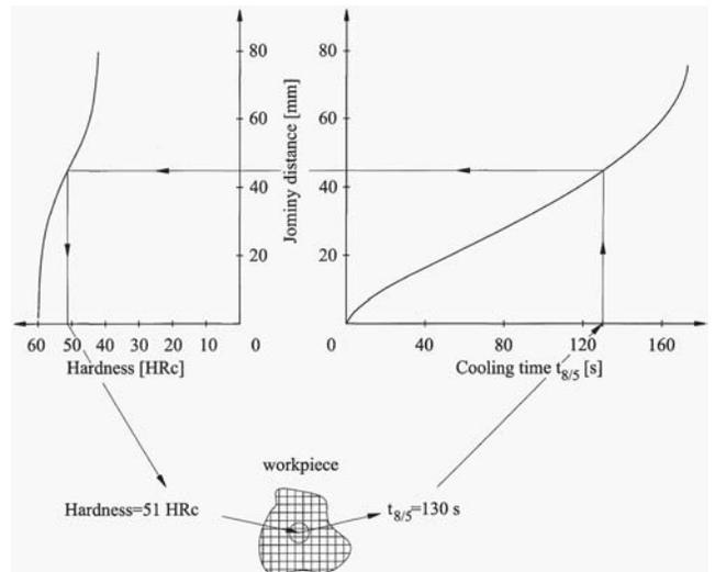
Fig. 1. Conversion of the cooling time  $t_{8/5}$  to the hardness
