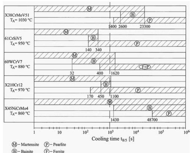
Fig. 2. Diagram of cooling times  $t_{8/5}$  of several different steels for tools and dies
