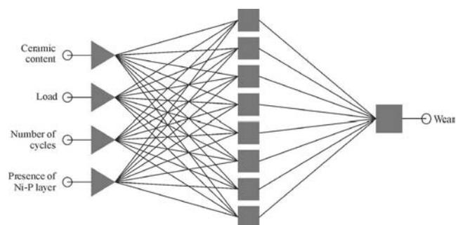
Fig 4. The scheme of neural network MLP 4-8-1 used modeling of tribological properties of composite materials
