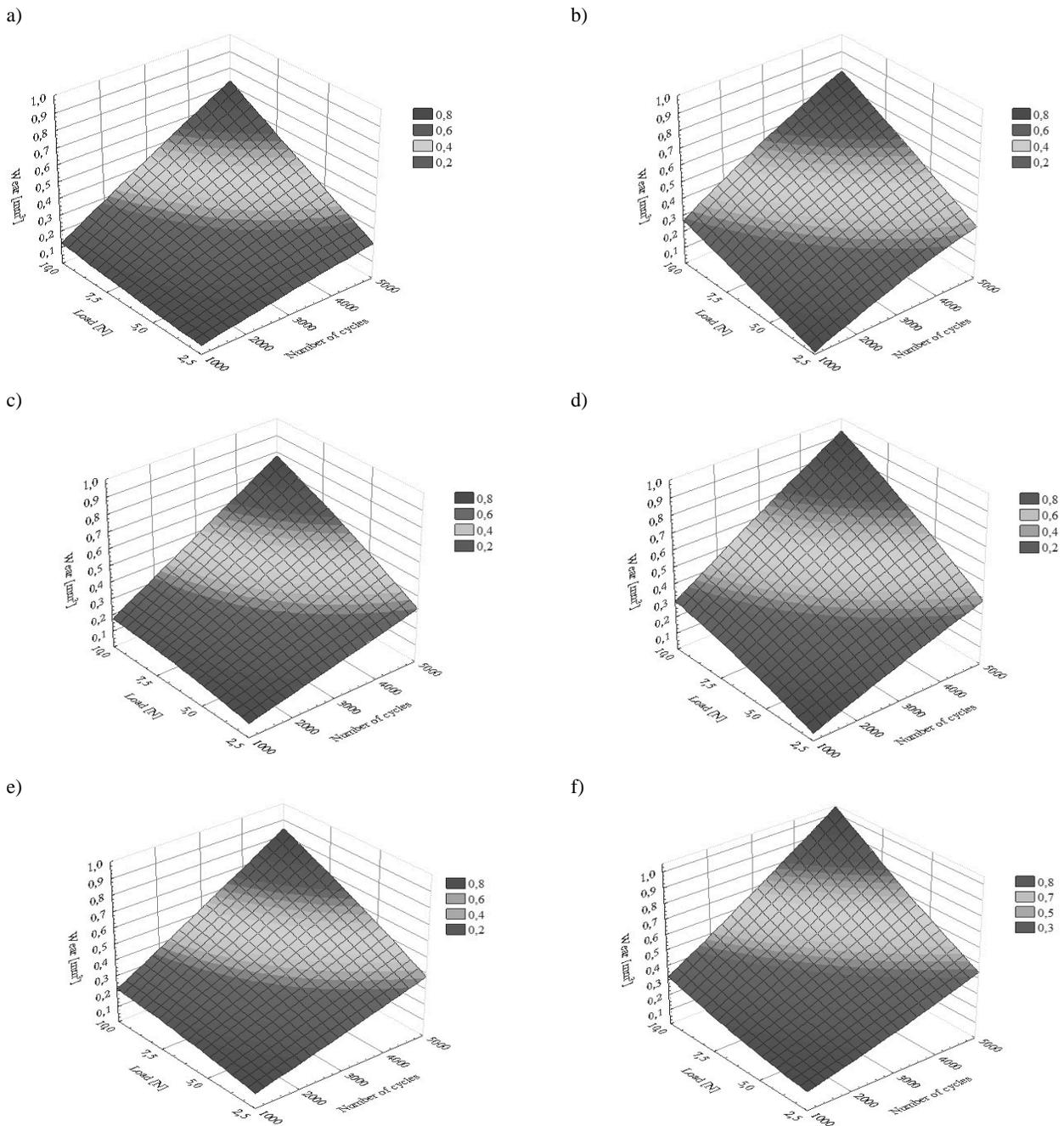
Fig. 5. Simulation of the load and number of cycles influence onto the abrasive wear of composite materials with volumetric portion of ceramic phase: a,b) 31%, c,d) 25% and e,f) 20%, (a, c, e - uncoated reinforcement, b, d, f - reinforcement coated by Ni)
