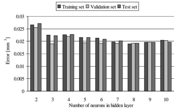
Fig. 3. The influence of neuron number in hidden layer on the network error
