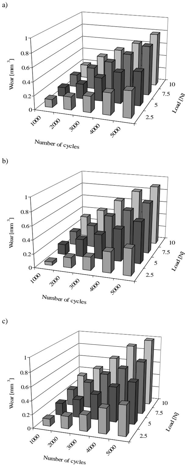
Fig. 2. The influence of load and friction distance on the wear of obtained composite materials with different ceramic content (reinforcement coated by Ni): a) 31%, b) 25% and c) 20%.
