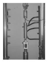
Fig. 14. A MTS test station for the evaluation of dynamic characteristics of the prototype MR damper
