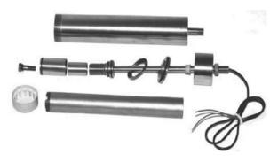
Fig. 2. Prototype MR Damper
